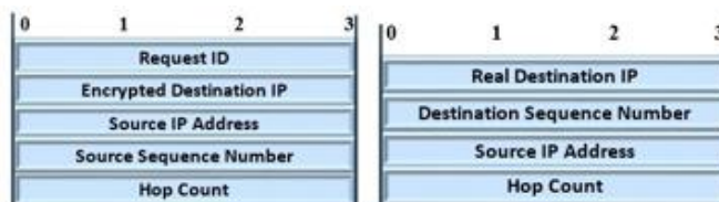
Figure 2 RREQ (Left) and RREP (Right) Packet Format of Red-AODV
