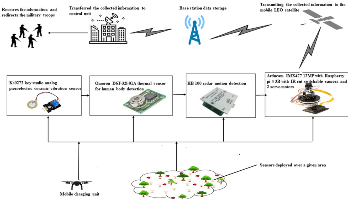
Figure 7 Framework Architecture for Border Surveillance System
