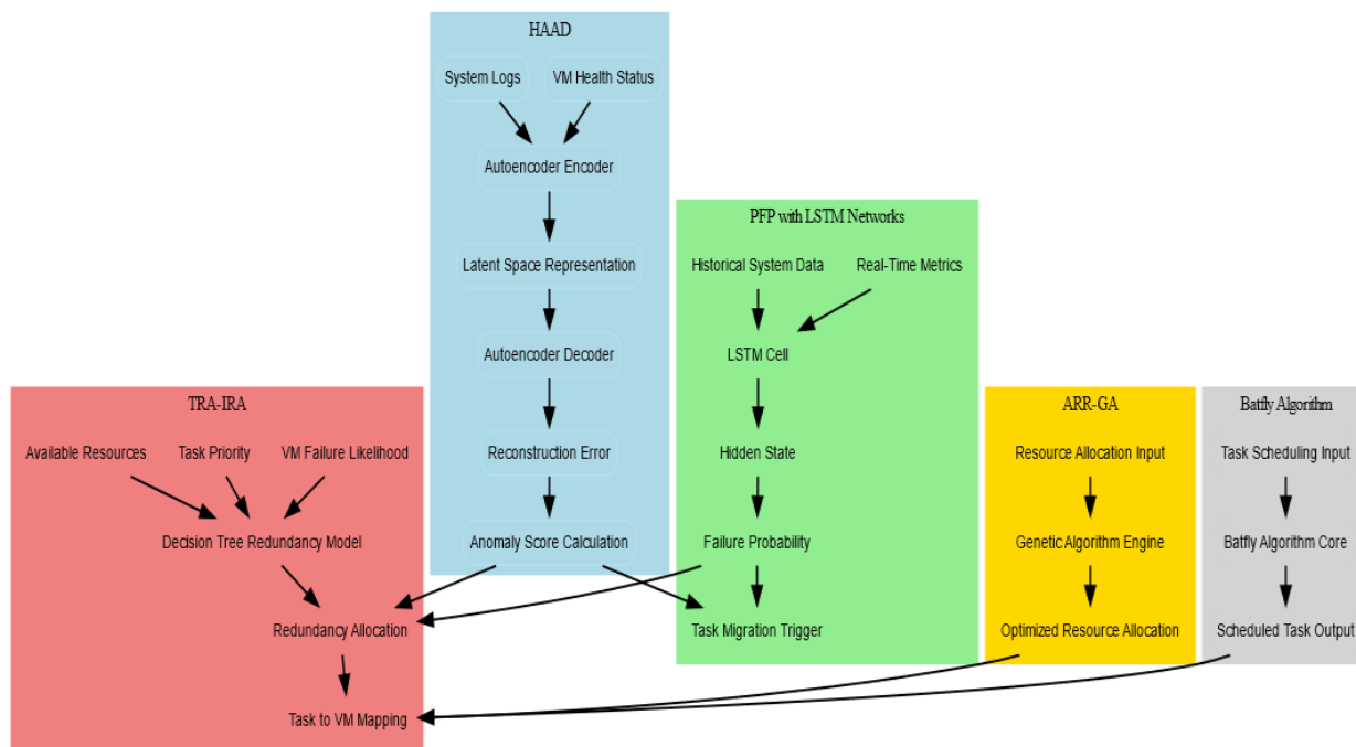
Figure 2 Model Architecture of the Proposed Fault Detection Process
